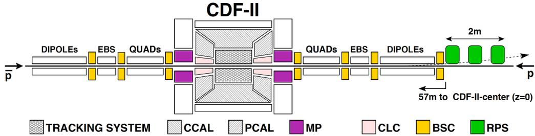
Fig. (1). Schematic plan view of the CDF II detector showing the tracking system and calorimeters (CCAL, PCAL), and forward components (MP, CLC, BSC, RPS); the BSC are electrostatic beam separators.
