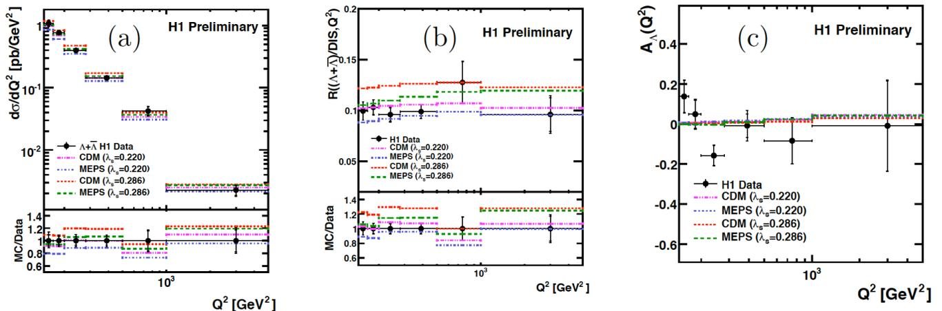
**Fig. (3).** The  $Q^2$  dependence of (a) differential  $\Lambda$  production cross section, (b) ratio  $R(\text{DIS})$  of  $\Lambda$  production to DIS cross section and (c) asymmetry  $A_\Lambda$  in comparison to RAPPAP (MEPS) and DJANGO (CDM) with two different values of  $\lambda_s$ . The inner (outer) error bars show the statistical (total) errors. The “MC/Data” ratios are shown for different Monte Carlo predictions. For the ratios the data points are put at one for comparison.
